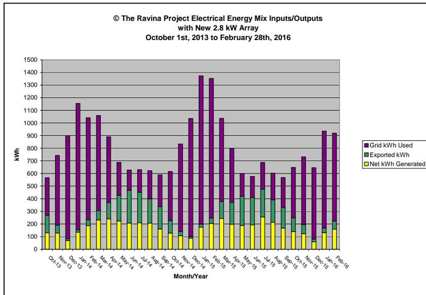
Let's unpack this chart above. It is identical to the previous chart with the energy use from natural gas deleted. This chart focuses on only electricity usage, generation and export. As you can see only in the summertime does the generation approach the amount of energy used from the Grid, marked as "Grid kWh Used" on the chart. We
