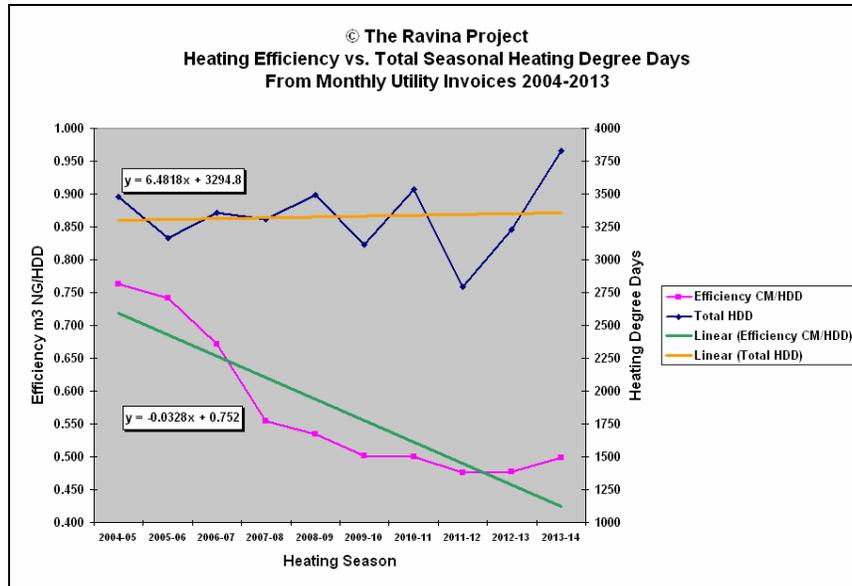
Let's unpack this chart. The left scale is the efficiency scale. Use it to read the magenta curve. On the right is the scale detailing the number of Heating Degree Days (HDD). Use it to read the blue line. The two straight lines give you an idea of whether the values of the two curves are increasing or decreasing. The heating seasons covered in the chart are listed on the bottom scale.
