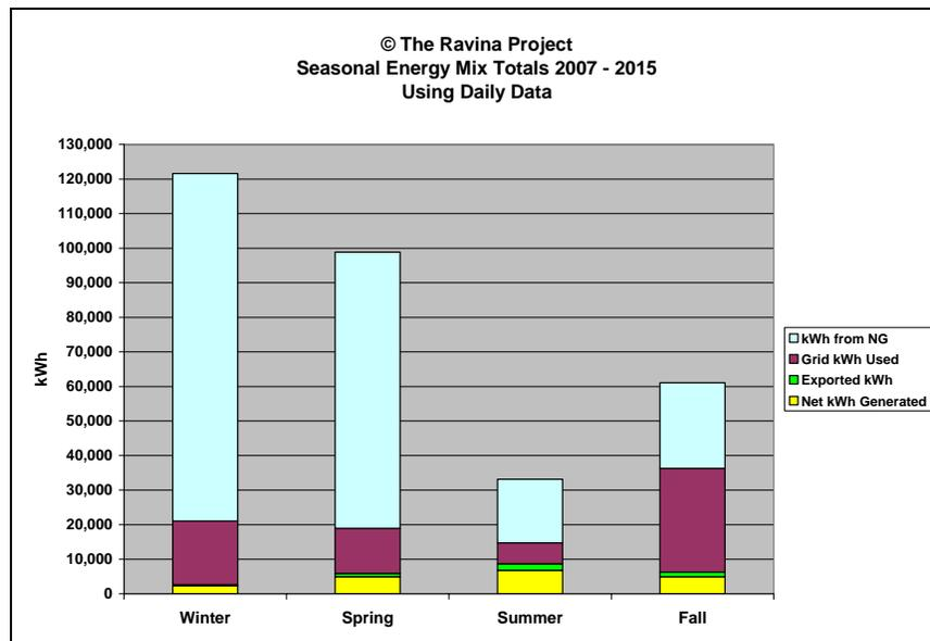
The yellow, 'Net kWh Generated' is the amount of energy generated by our solar panels that we used to energize our household. The green 'Exported kWh' represents the energy we pushed back to the Grid. The violet 'Grid kWh Used' represents the amount of Grid energy we used. And lastly, the blue represents the amount of energy we used from natural gas converted to kWh with the conversion factor of one cubic meter of natural gas is equal to 10.35 kWh at STP (Standard Temperature and Pressure).
