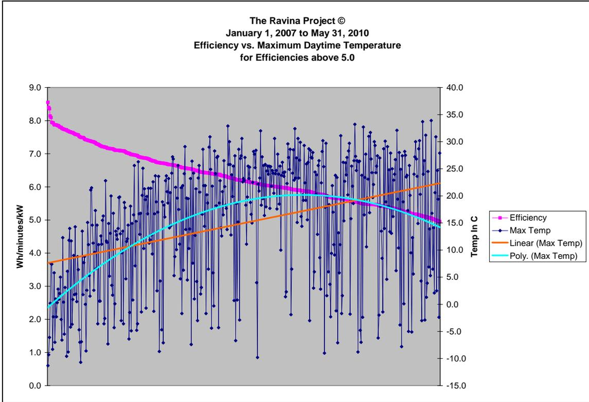
As the curves progress from right to left in the chart the weather becomes less and less a factor as a higher percentage of days have better generation conditions. The relationship between RSES numbers and maximum daytime temperatures becomes apparent as a strongly negative correlation especially when the RSES number gets above 6.0. This transition becomes apparent around the maximum temperature of between 20 and 25 degrees C.
