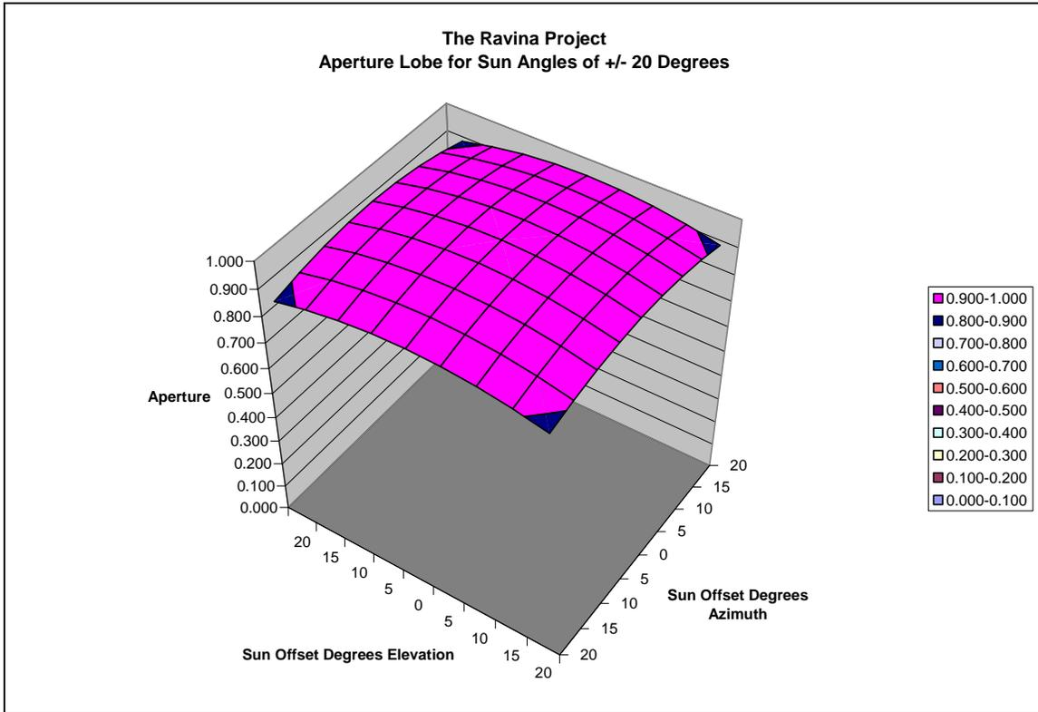
This graphic shows the two axis offset of +/- 20 degrees from Normal. The aperture is at least .900 for the vast majority of the offset angles. This is a large rectangle in the sky for the sun to be inside of all day long. The sun can move square root (3200) or 56 degrees across the sky and still be within the .900 aperture for the overwhelming majority of that trip.
