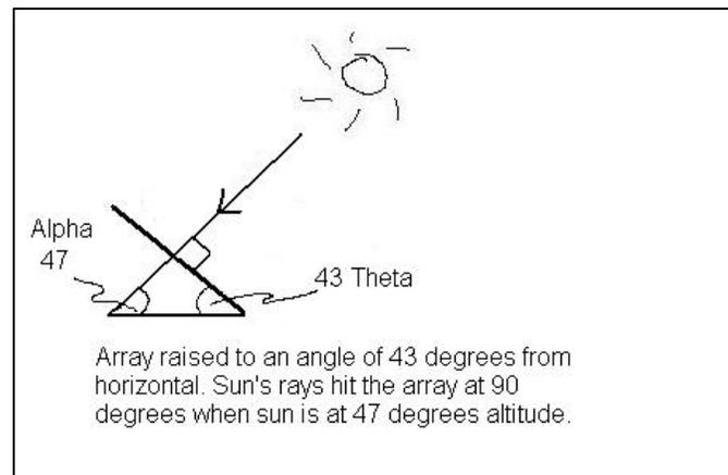
alpha decreases by 17 degrees to become 30, the right angle must increase by 17 degrees to compensate. The sun's ray hits at an offset of 17 degrees from normal on the vertical axis. From the argument above we know that the effective vertical dimension of the array varies as the cosine of the offset. The vertical dimension becomes  $\text{COS}(17)$  or .96m.
