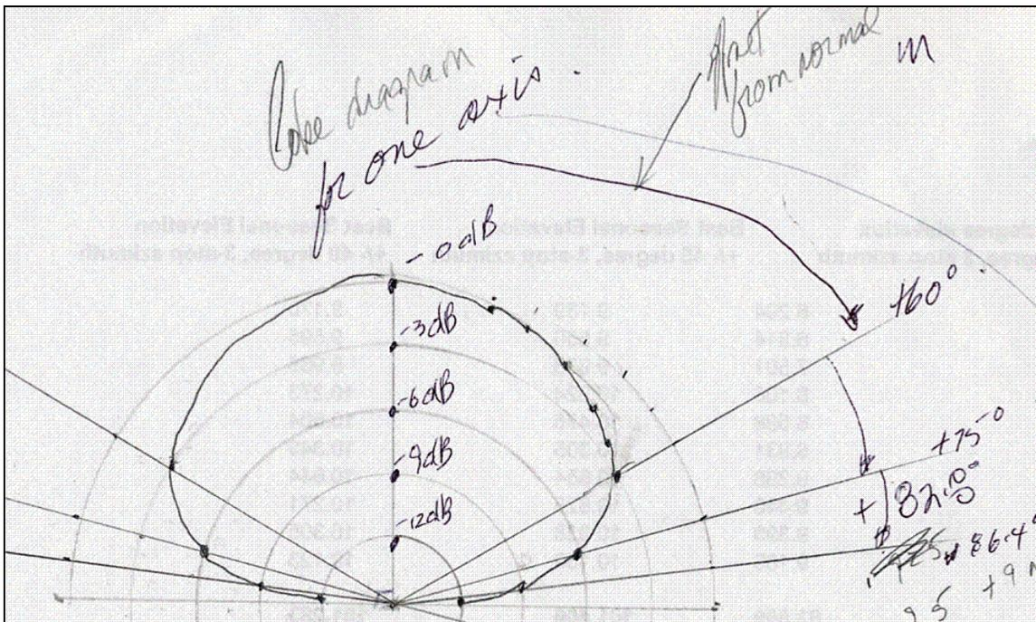
The concentric circles are measured in 3.0 dB intervals. We can see that at an offset of 60 degrees the power has fallen by half or minus 3.0 dB. This is the power plot of our array of solar panels. From my point of view it sure looks like the plot of a radio antenna. Maybe this paradigm, that of treating the receiving characteristics of an array of solar panels as a radio antenna, is not too far from being right on.
