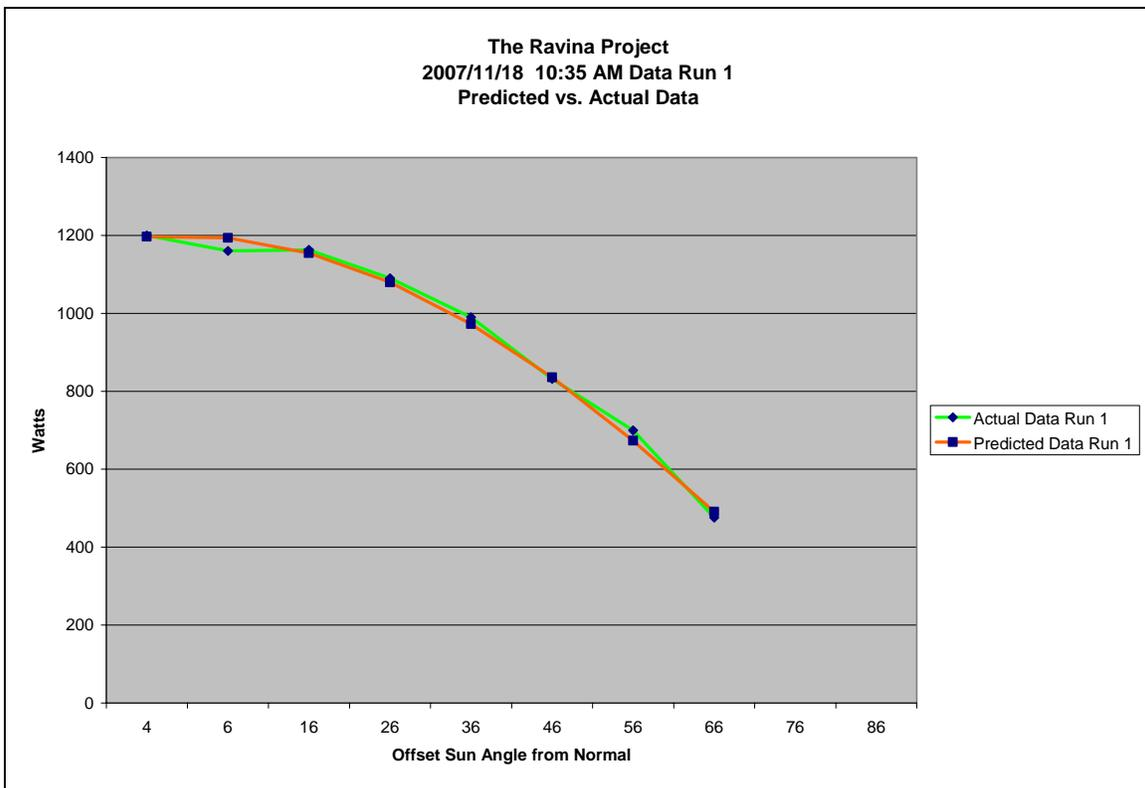
Sun power changes as a result of azimuth changes are not involved. The measurements were taken in such a short period of time that sun movement on the azimuth is minimal. This data reflects only power changes that are the result of changes in the angle of the sun upon the collecting surface.
