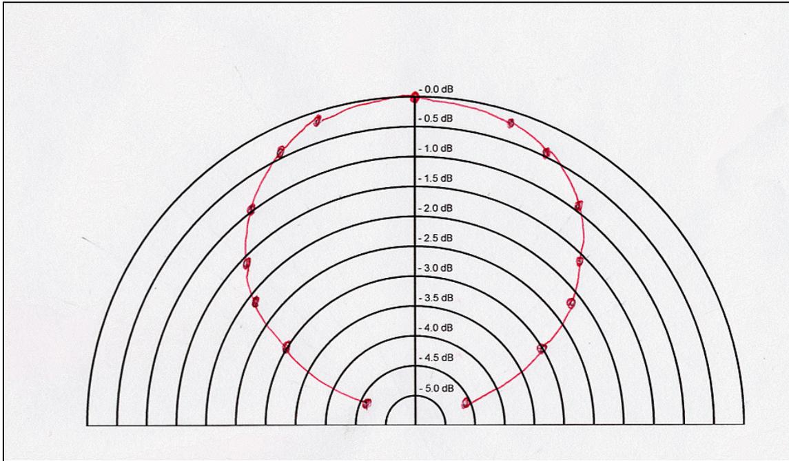
**Solar Array Power Roll Off Pattern**
