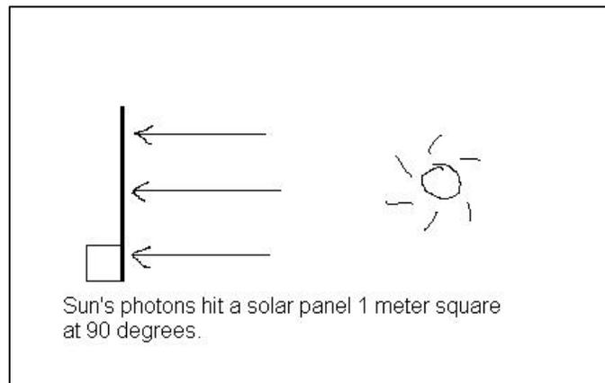
The point of view is from the end of the array. The sun’s rays (photons) hit the array in parallel lines. One of our assumptions in the paper mentioned above is that when solar radiation hits the aperture of the array at 90 degrees, or Normal, the number of photons intercepted is at a maximum. The signal power received is at a maximum. The solar array will generate maximum power in this orientation to the sun.
