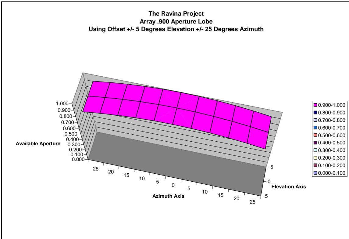
If the array surface were reduced to a point, a rectangle one meter away would have 17.5 cm on one axis and 93.3 cm on the other. This patch in the sky would have a surface area of about 1,632.8 square cm.
