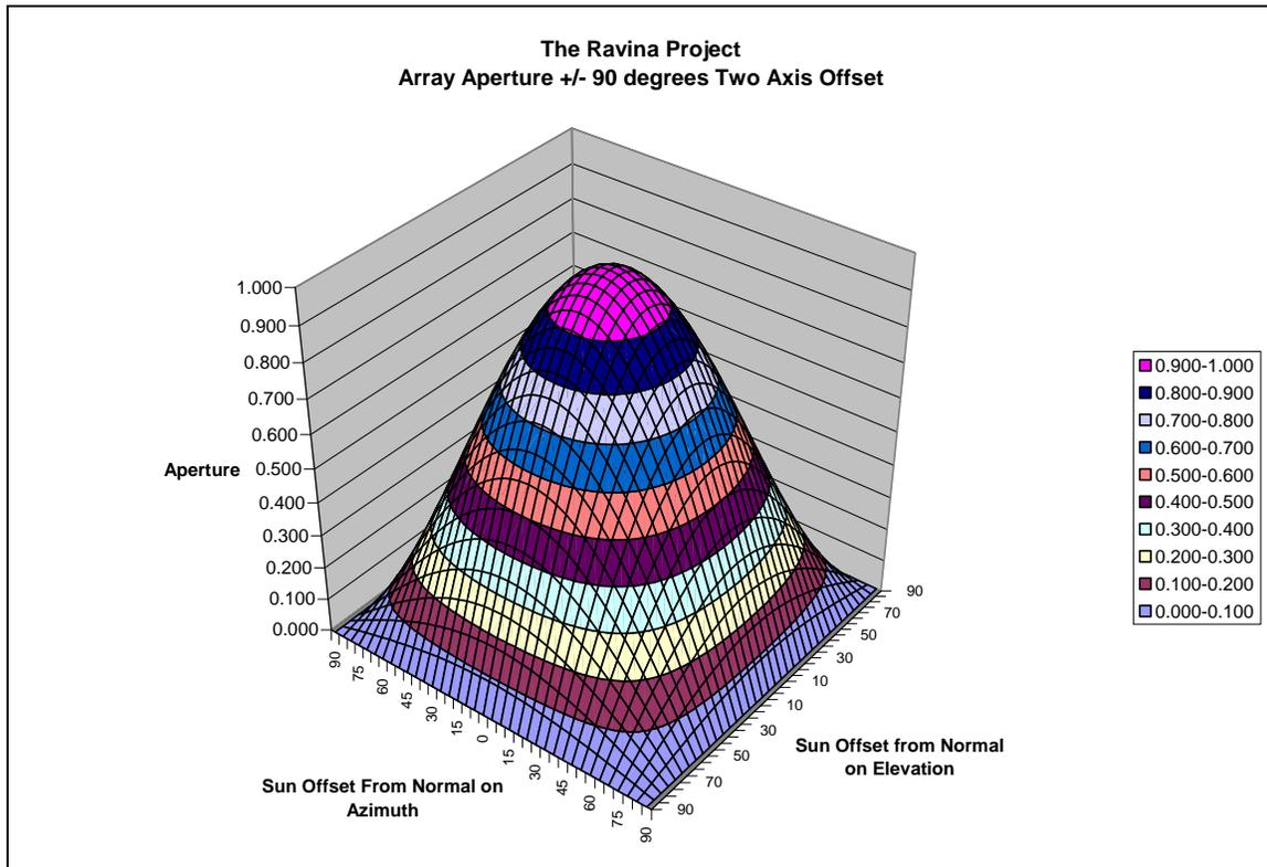
This graph represents the power receiving lobe of our array constructed according to our model of array evaluation.
