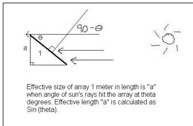
The angle theta approaches zero as the dimension 'a' approaches zero. As the angle theta approaches 90 degrees, the dimension 'a' approaches unity which is the physical length of the array. This approach to calculating an effective dimension of the array can work for both the array's effective width and its effective height. This allows for the calculation of the array's effective aperture.
